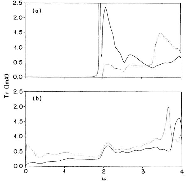
FIG. 4. Spectral function  $\text{Tr Im}\chi$  for the same parameters as Fig. 3. The sharp excitonic features in the charge channel at  $\mathbf{q}=0$  have been broadened by adding a small imaginary part to the frequency  $\text{Im}\omega=10^{-3}$ . Solid lines,  $\chi_\rho$ ; dashed lines,  $\chi_\sigma$ ; (a)  $\mathbf{q}=(0,0)$ ; (b)  $\mathbf{q}=(\pi,\pi)$ .
