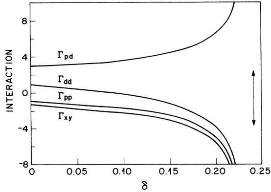
FIG. 16. Effective interactions between particles on near-neighbor sites as a function of doping, for the same parameters as Fig. 15. The arrow marks the CTI.
