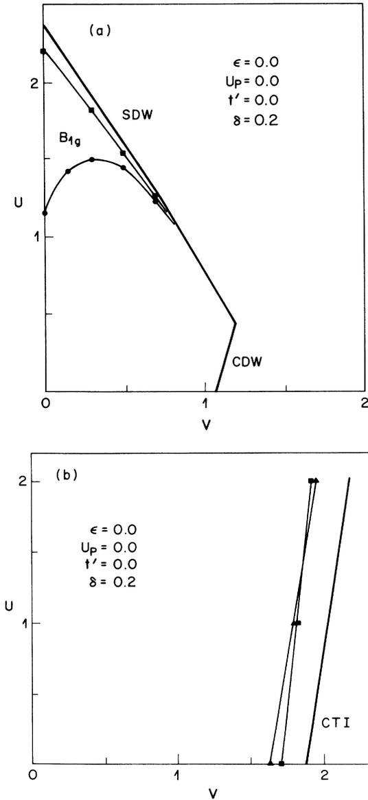
FIG. 12. Instabilities of the normal state for  $\epsilon=0$ ,  $t'=0$ , and  $U_p=0$  with (a) or without (b) the inclusion of intraband coupling terms in the evaluation of the effective interaction. Superconducting instabilities are shown for  $T_c=10^{-4}$ , in three different symmetries: Circles,  $B_{1g}$  ( $d_{x^2-y^2}$ ); squares,  $A_{1g}$  ( $s$ ); triangles,  $B_{2g}$  ( $d_{xy}$ ).
