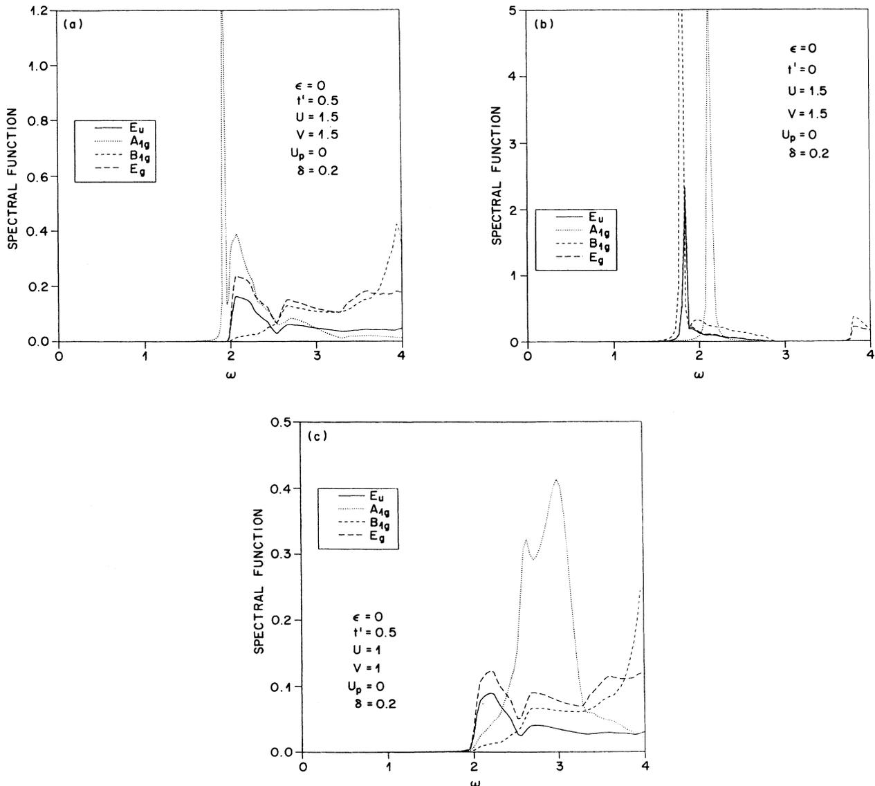
FIG. 5. Spectral function for charge excitations at  $\mathbf{q}=(0,0)$  separated into symmetry components, for different values of the parameters.
