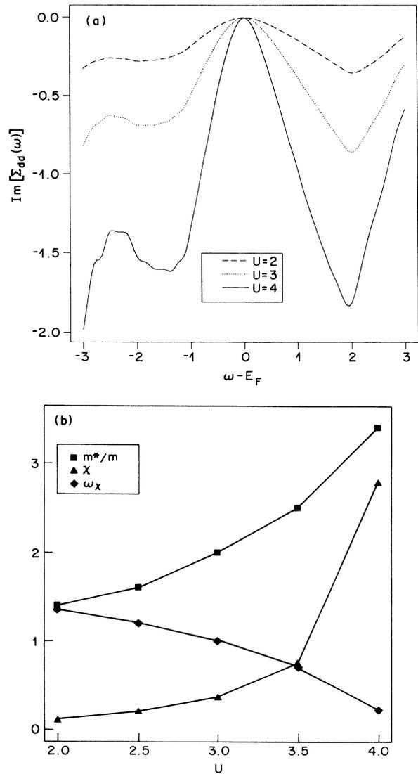
FIG. 11. (a)  $\text{Im}\Sigma_{dd}(\omega)$  for the same parameters as Fig. 10(a); (b) effective mass renormalization on the Fermi surface (squares); peak position of the susceptibility (triangles); and peak frequency ( $\times 10$ ) of the susceptibility peak (diamonds).
