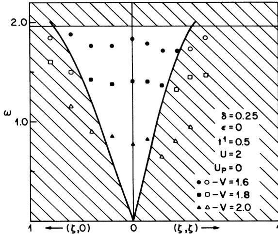
FIG. 6. Dispersion relation for the charge-fluctuation collective modes for three different values of  $V$ ; hatched areas mark the continuum of particle-hole excitations; solid symbols represent undamped excitations (outside the particle-hole continuum); modes which remain underdamped in the continuum are shown by open symbols.
