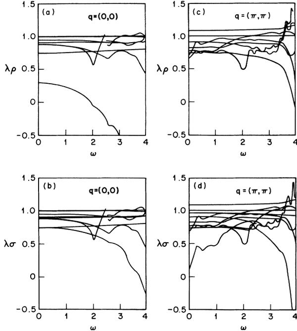
FIG. 3. Real part of the eigenvalues of the non-local charge [(a) and (c)] and spin [(b) and (d)] susceptibilities  $\lambda_{\rho,\sigma}(\mathbf{q},\omega)$  from the solution of Eq. (4). Parameters are  $U=1.5$ ,  $V=1.5$ ,  $U_p=0$ ,  $\epsilon=0$ ,  $t'=0.5$ . (a) and (b),  $\mathbf{q}=(0,0)$ ; (c) and (d),  $\mathbf{q}=(\pi,\pi)$ .
