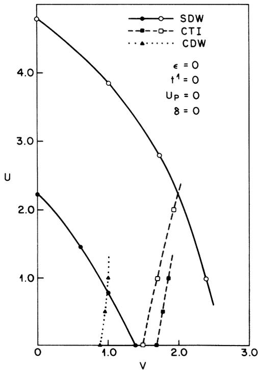
FIG. 7. Phase diagram as a function of  $U, V$  at a doping  $\delta=0.2$ . In all cases, we mark the instabilities of the metallic phase, even though some of the phases may not be accessible on account of preemption by other transitions. Solid (open) symbols are the results without (with) second-order self-energy corrections.
