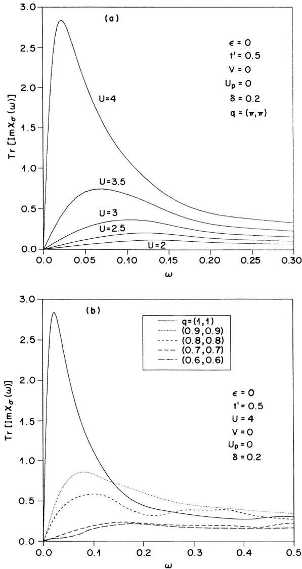
FIG. 10. Spin susceptibility  $\text{Tr} \text{Im}\chi_\sigma(\mathbf{q}, \omega)$ : (a) for  $\mathbf{q}=(1,1)$  as a function of  $U$ ; (b) for  $U=4$  as a function of  $\mathbf{q}=(\xi\xi)$ . The SDW instability sets in at  $U=4.15$  for these parameters.
