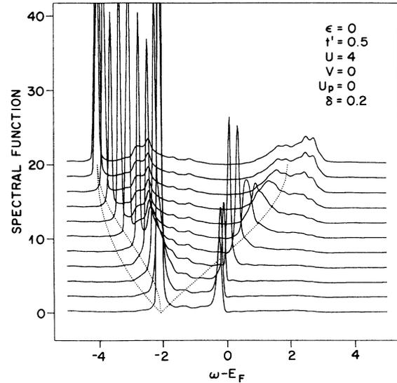
FIG. 8. Electron spectral function as a function of energy at fixed momenta along  $\mathbf{k}=(\zeta, \zeta)$ . The dotted line shows the dispersion relation for the single-particle Hamiltonian. Energies are measured relative to the Fermi energy.
